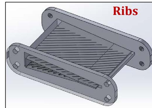
Excessive Pressure Drop and Mediocre Cooling ☹️
